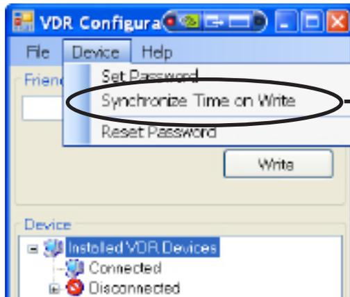
If the clock must be resynchronized, the Configuration Tool can be set to do this upon the next VDR Configuration Write event.
