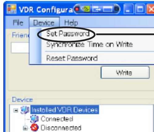
Use the top Device menu to select “Set Password” to change an existing known password. An “Enter New VDR Password” pop-up window appears. The “Set Password” function does not erase existing data.
