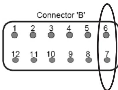
For each seat location (Example: Seat 6) the seat belt and the seat occupancy switch positions on the connector line up vertically
