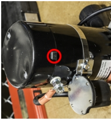
INCORRECT VENT HOLE ORIENTATION ROTATE MOTOR COVER 180°
