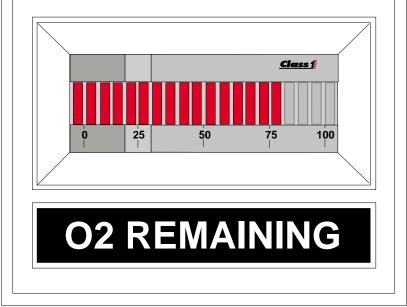
The *Class1* Oxygen Remaining Display is designed to provide operators with a visual indication of Oxygen remaining and an audible warning when there is less than 20% oxygen remaining. The audible warning is inactive whenever the pressure is below 50 PSI so that it will not sound when the supply is turned off.
