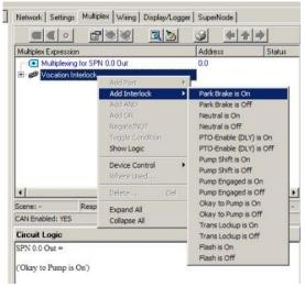
Figure 17. Applying vocation inputs.
