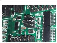
Figure 11. Input/output selection jumpers.
