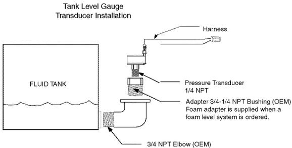
Mount the pressure transducer (sensor) vertically to insure an accurate reading and to reduce the possibility of sensor port contamination.
