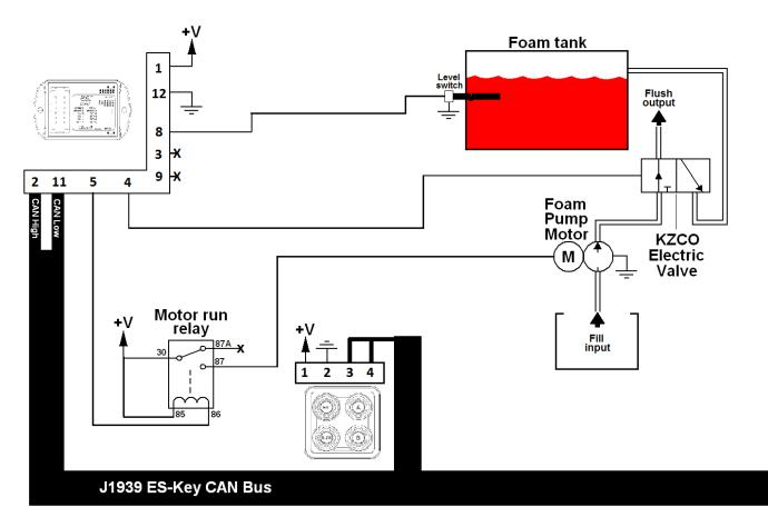
Figure 6-1: Typical Single Tank Electrical Schematic Overview
