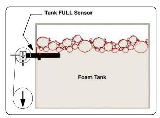
Tighten the sensor having the "arrow" on the base of the hex pointing down.
