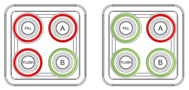
Figure 2-4: Dual Tank Configuration (Tank A selected left, Tank B selected right)
