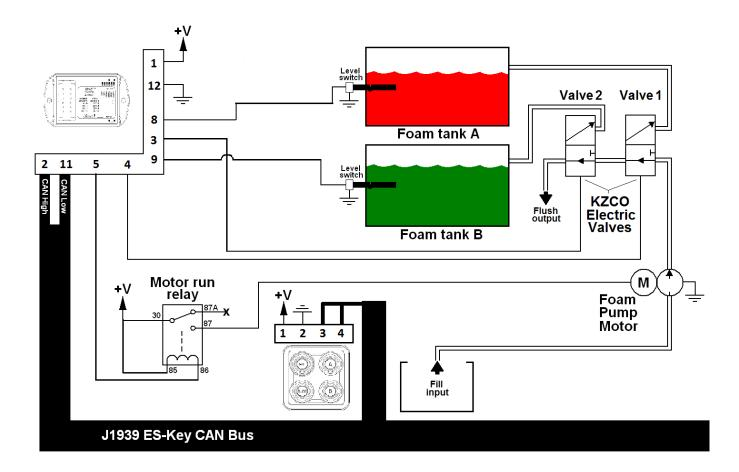
Figure 6-2: Typical Dual Tank Electrical Schematic Overview - Optional
